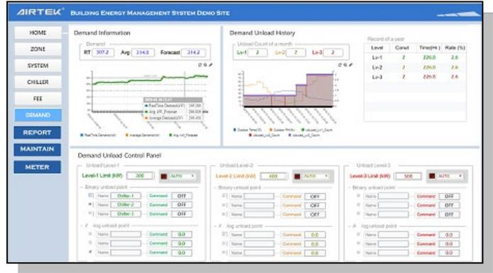
● 建築能源管理系統支援 (Building Energy Management system support(BEMS))
